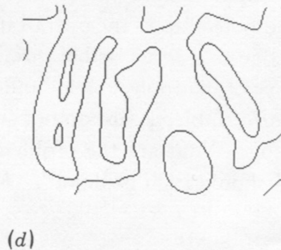
FIGURE 3. The image (a), which is 320 \times 320 pixels, has been convolved with \nabla^2 G , a centre-surround operator with central excitatory region of width 2\sigma = 6, 12 and 24 pixels. These filters span approximately the range of filters that operate in the human fovea. The zero-crossings of the filtered images are shown in (b), (c) and (d). These are the precursors of the raw primal sketch. (From Marr & Hildreth 1979, figure 6).
